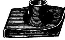
8377.....60Ea 5/16-18 Screw Panel Range .060"-.090", Ctr Of Hole To Edge 9/16"
